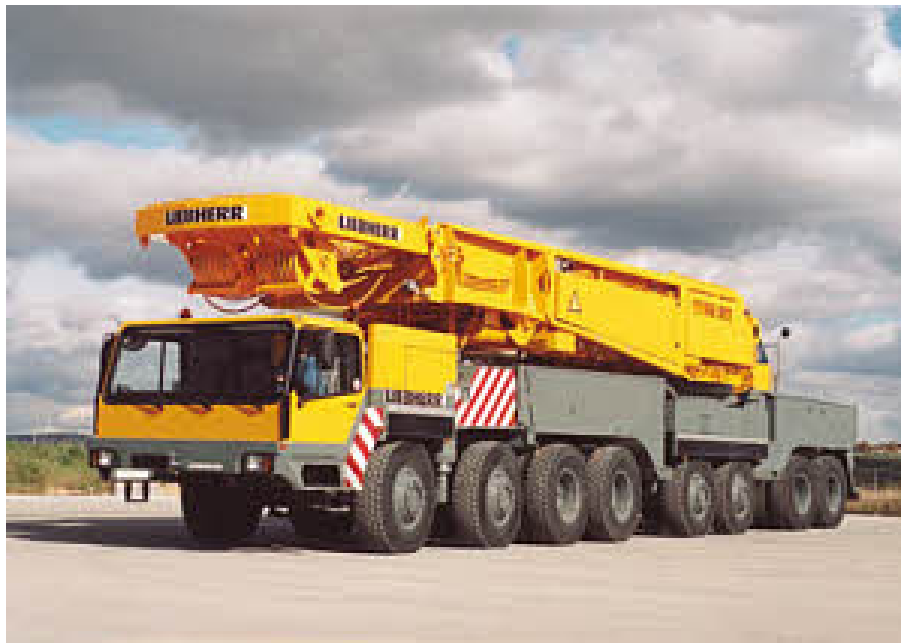
Figure 4.4-5: Example of a Hydraulic Road-Going Crane (Hydraulic Mobile Crane LG1550)
