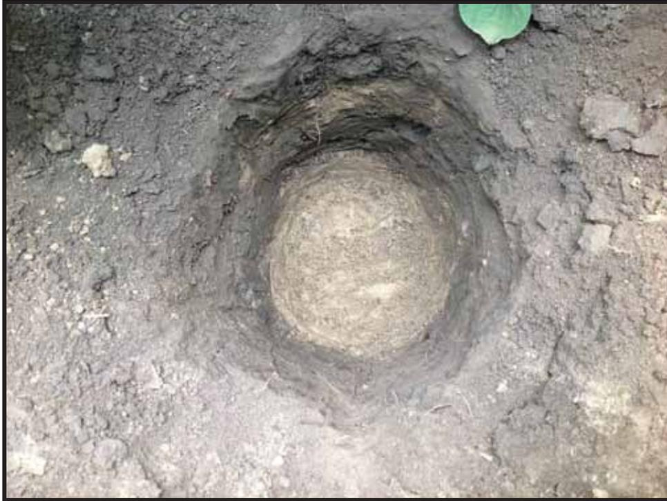
**Image 21: View of Typical Test Pit Excavated 5 cm into Subsoil at GSH1023**
