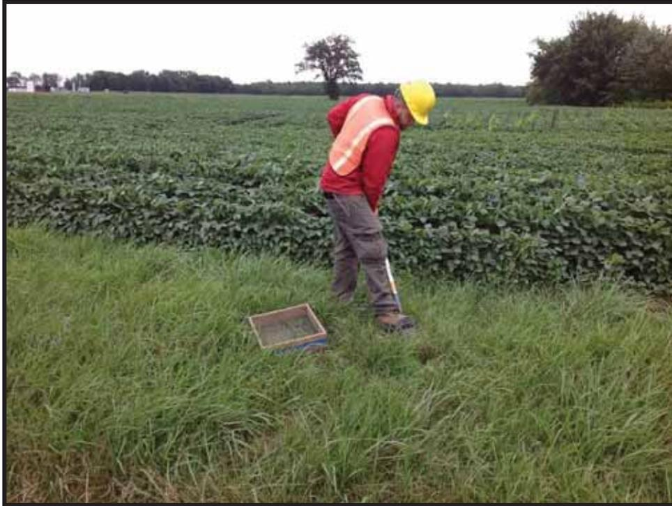
**Image 15: View of Crewmember Test Pitting to Confirm Disturbance at GSH1022/2176**
