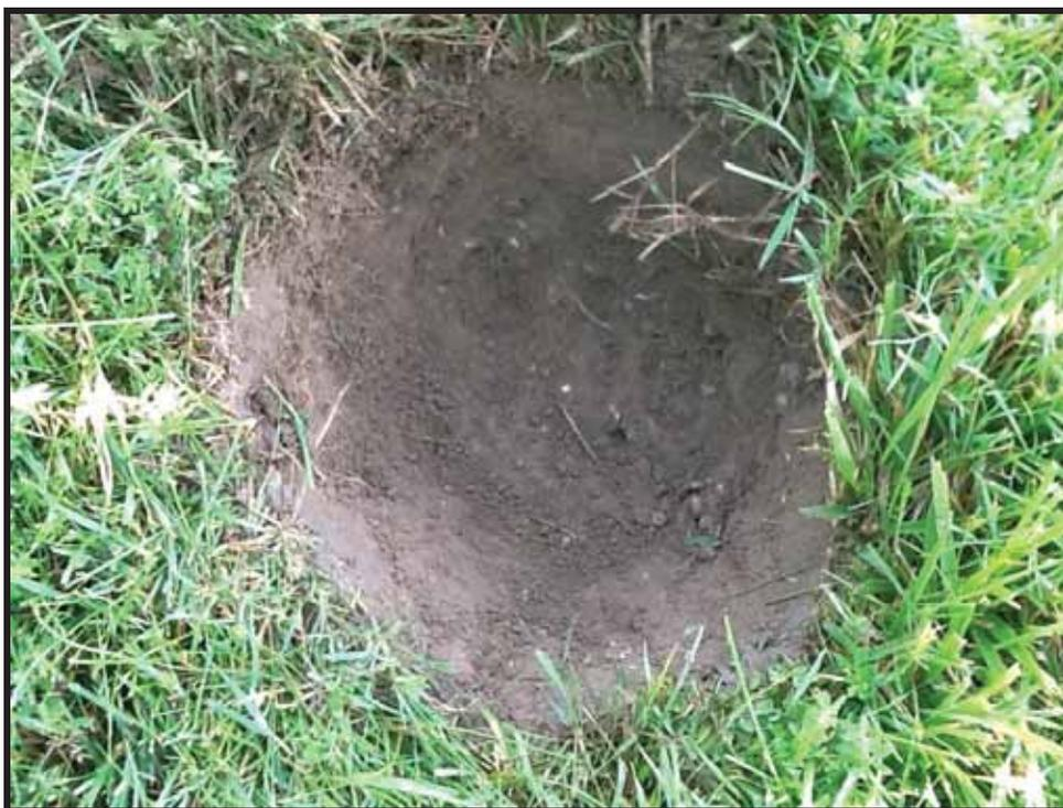
**Image 46: View of Disturbed Test Pit at GSH1043 (North)**
