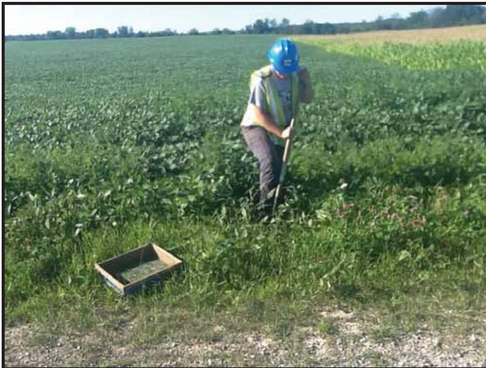
**Image 86: View of Crewmember Test Pitting to Confirm Disturbance at GSH1118**
