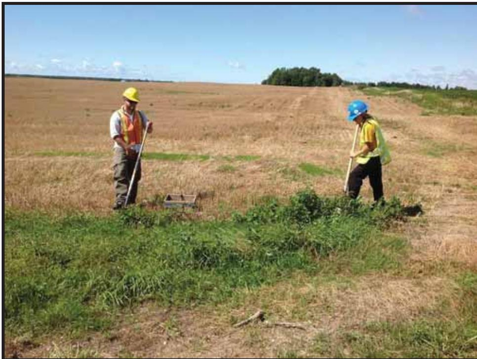
**Image 72: View of Crewmembers Test Pitting at a Maximum Interval of 5 m at GSH1072**
