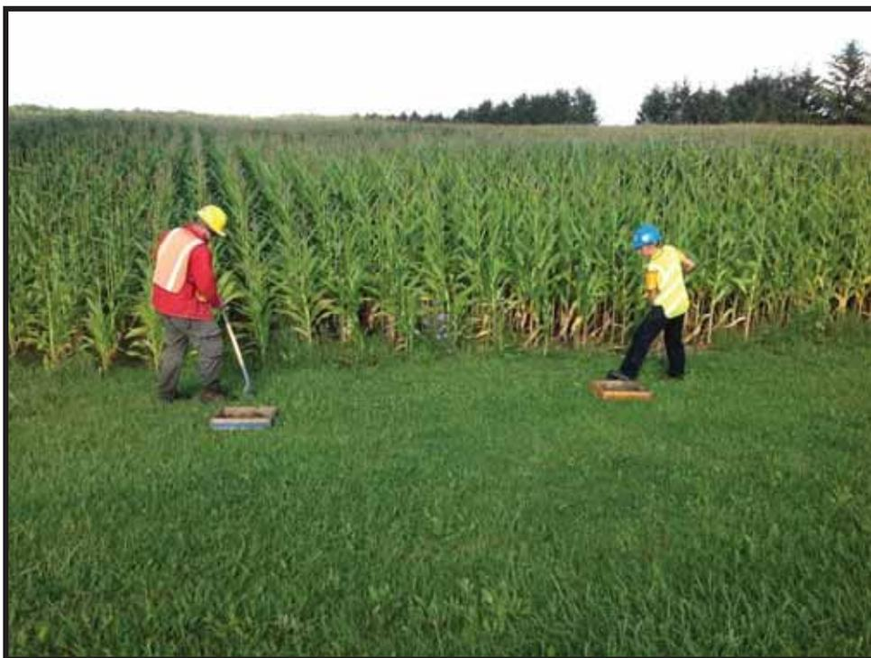
**Image 114: View of Crewmembers Test Pitting to Confirm Disturbance at GSH1507**
