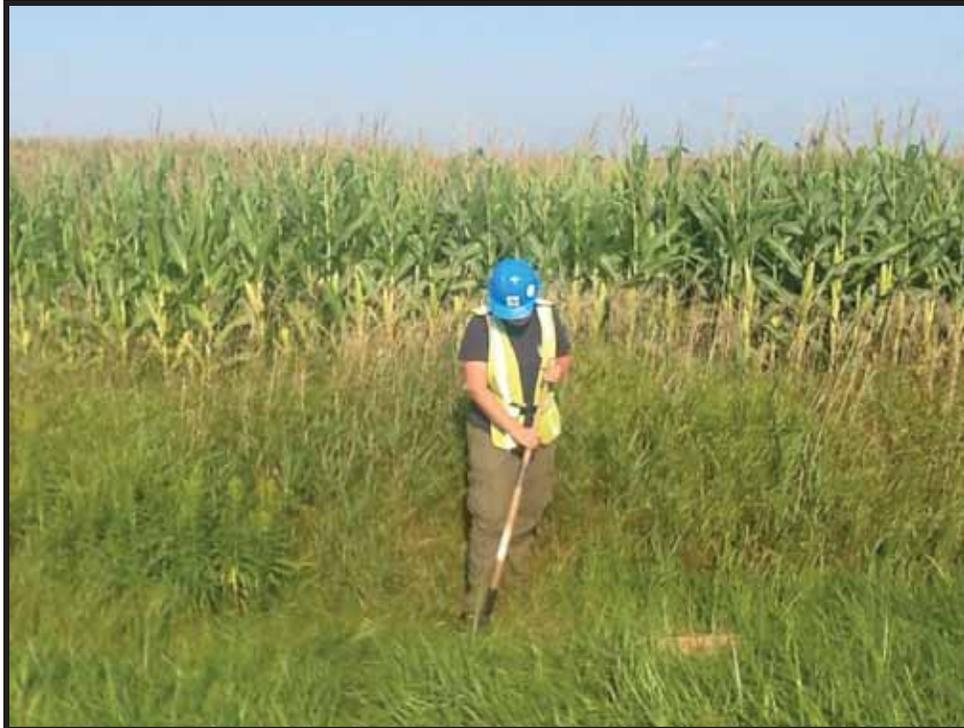
**Image 55: View of Crewmember Test Pitting to Confirm Disturbance at GSH1061**
