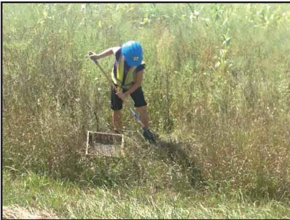
**Image 42: View of Crewmember Test Pitting to Confirm Disturbance at GSH1040**
