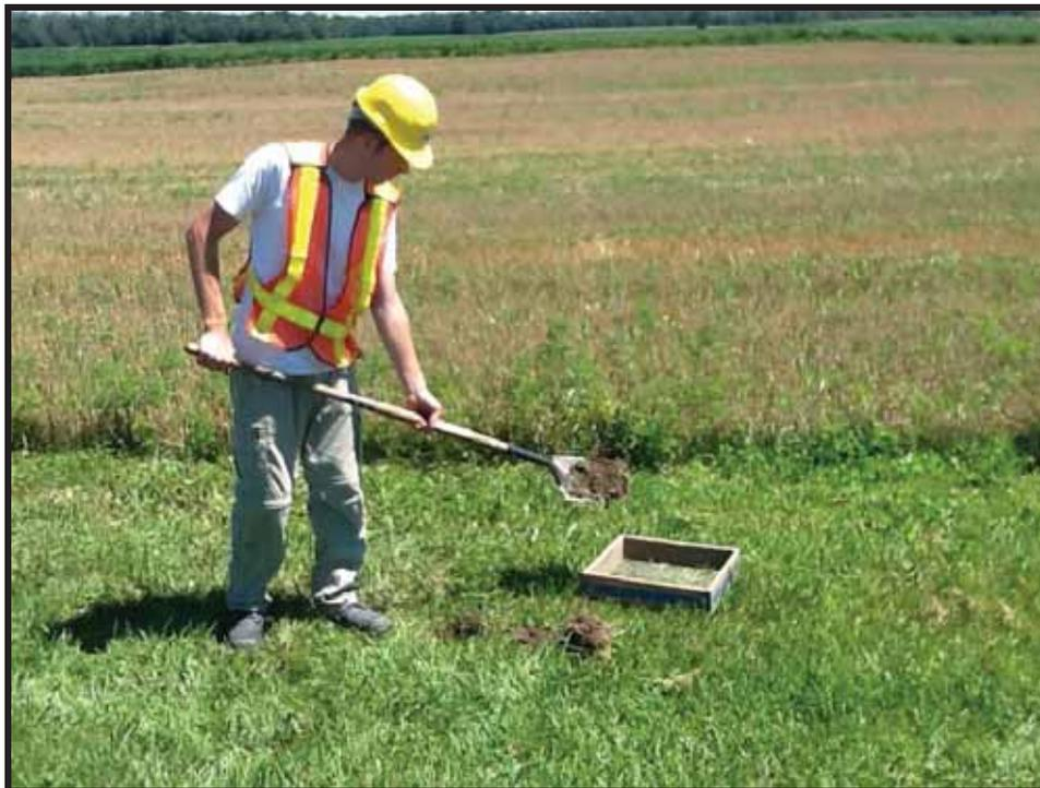
**Image 100: View of Crewmember Test Pitting to Confirm Disturbance at GSH1481**
