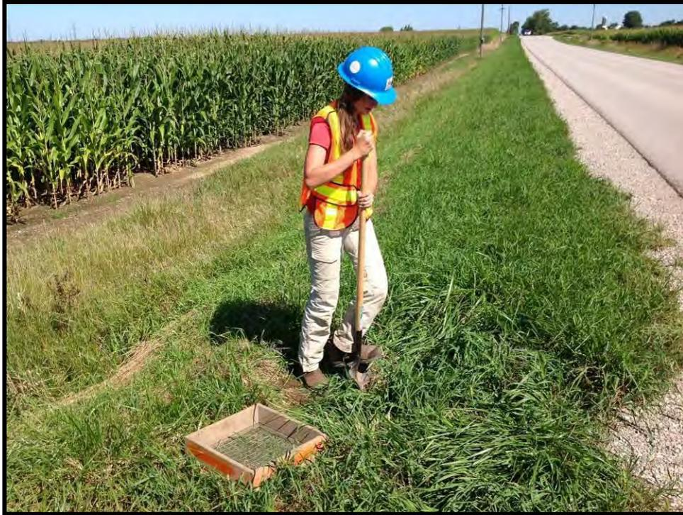
**Image 155: View of Crewmember Test Pitting to Confirm Disturbance at GSH2043**
