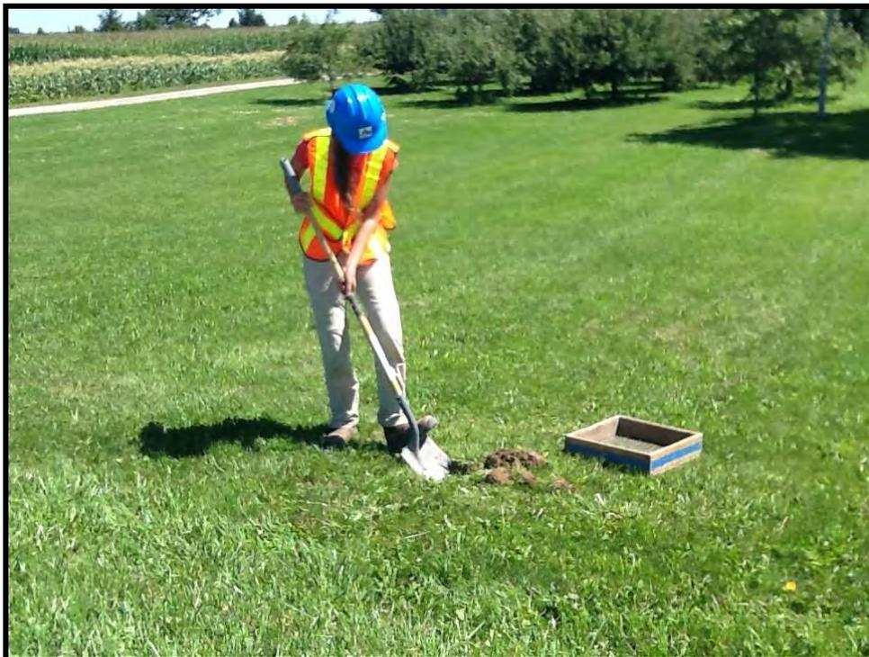
**Image 158: View of Crewmember Test Pitting to Confirm Disturbance at GSH2046**
