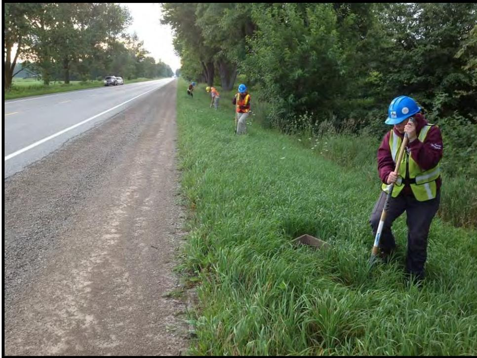
**Image 165: View of Crewmembers Test Pitting to Confirm Disturbance at GSH2099**
