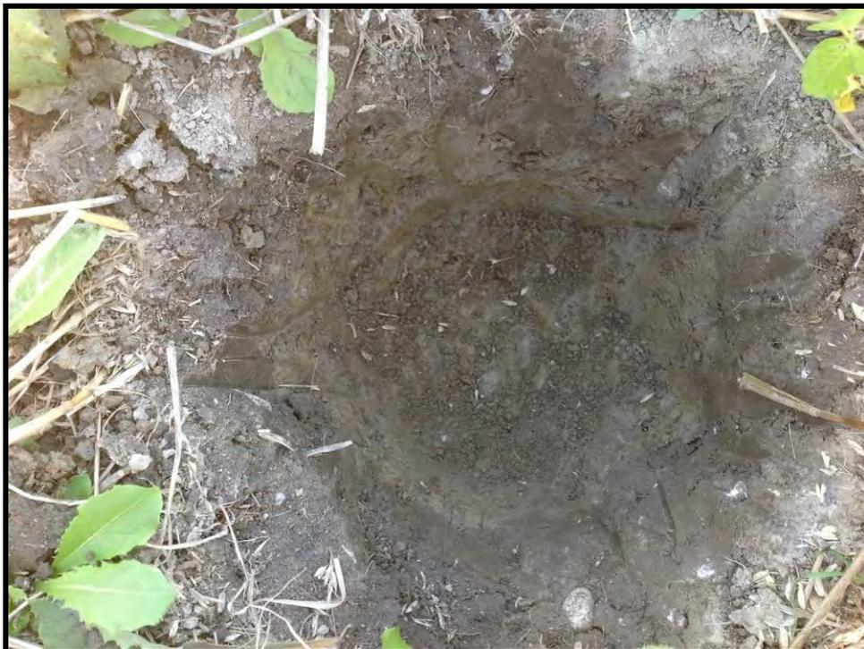
**Image 84: View of Typical Test Pit Excavated 5 cm into Subsoil at GSH1095**
