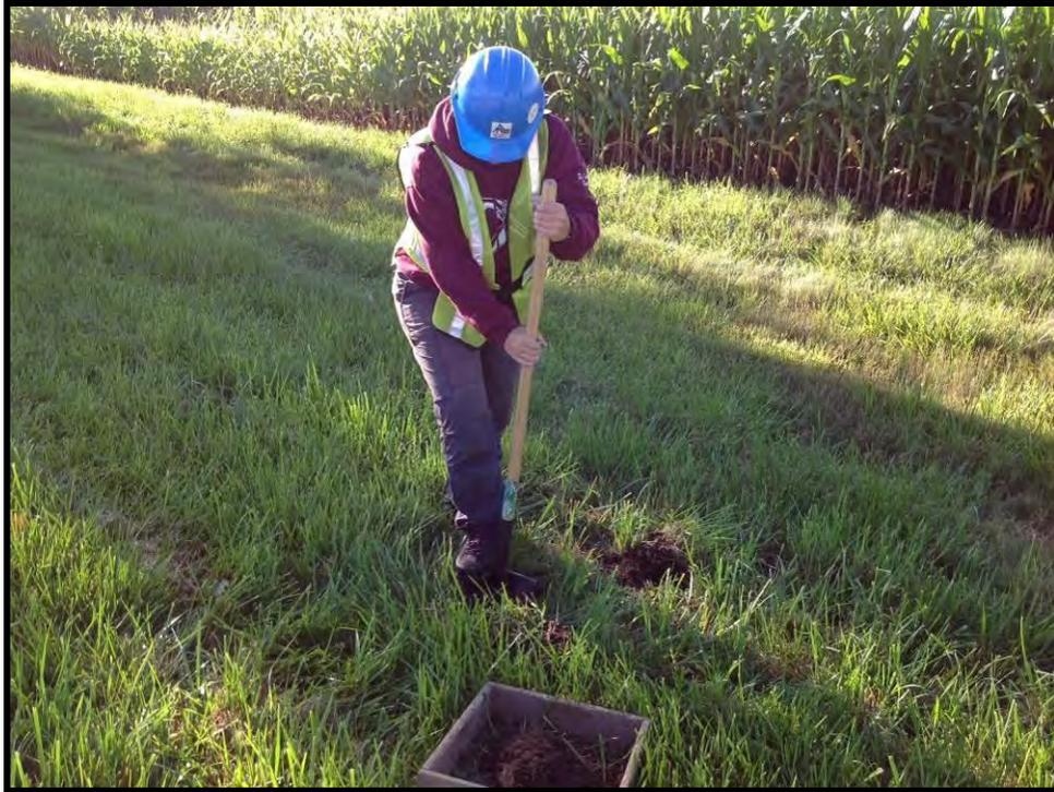
**Image 7: View of Crewmember Test Pitting to Confirm Disturbance at GSH1012
