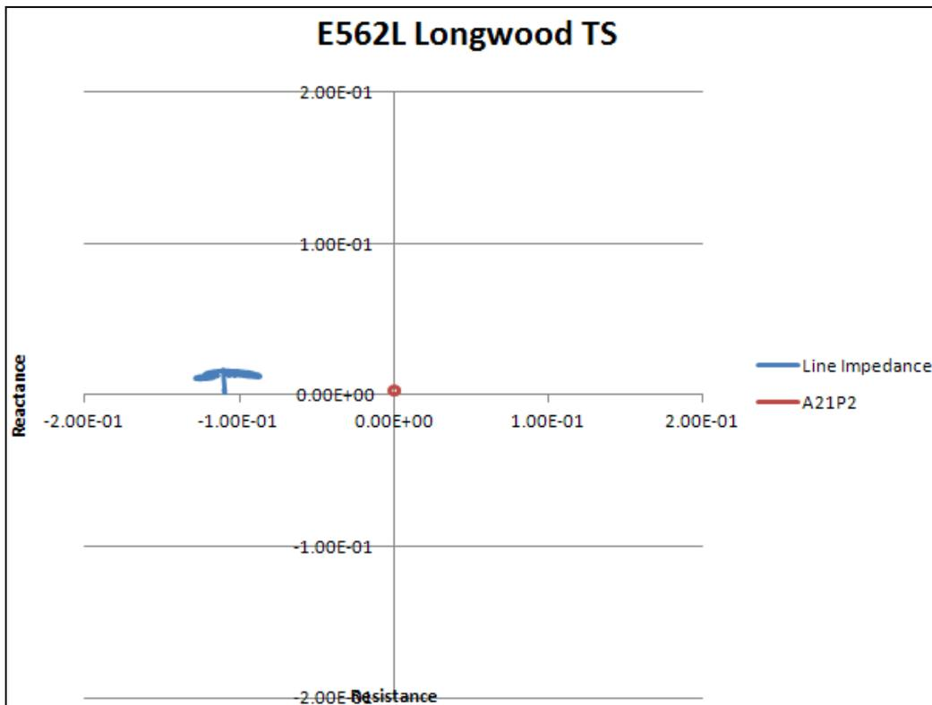
Figure 12: E562L @ Longwood trajectory for a LLG fault on B560V and B561M at Willow Creek Junction
