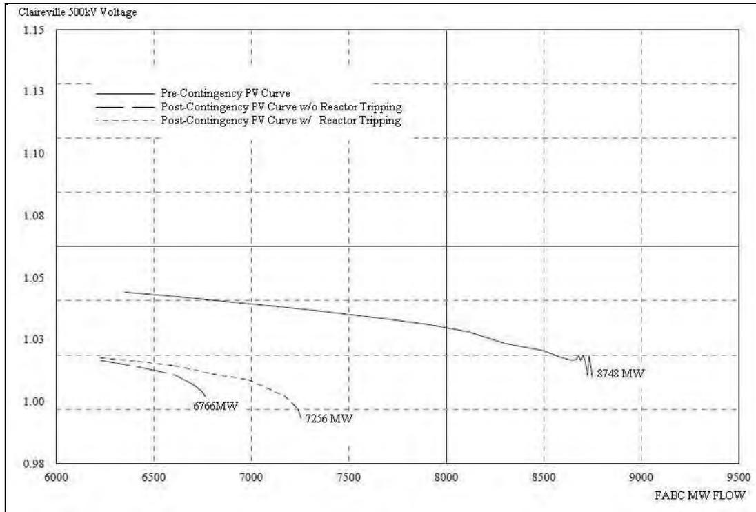
**Figure 3: Voltage performance at Claireville 500kV vs. FABC transfer**
