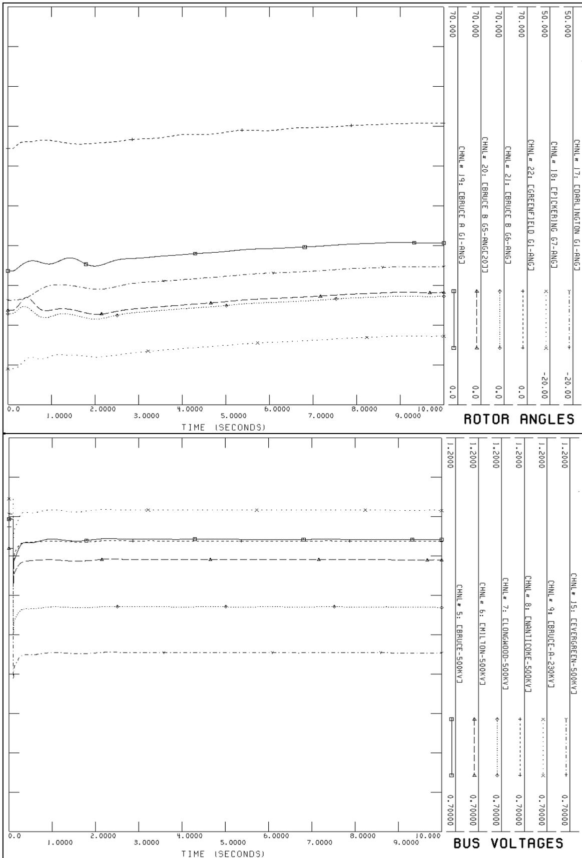
Figure 7: Parkhill 121 kV - Un-cleared 3 phase fault
