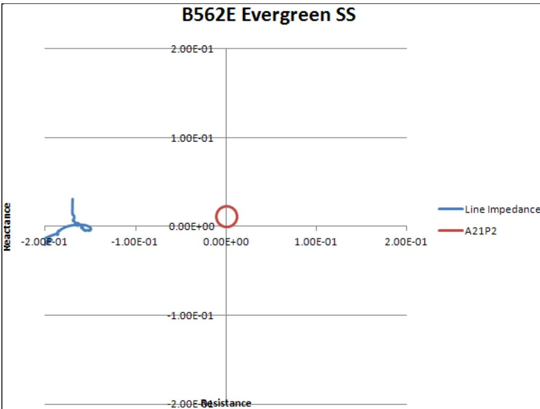
Figure 18: B562E @ Evergreen trajectory for a 3 phase fault on A563L at Longwood
