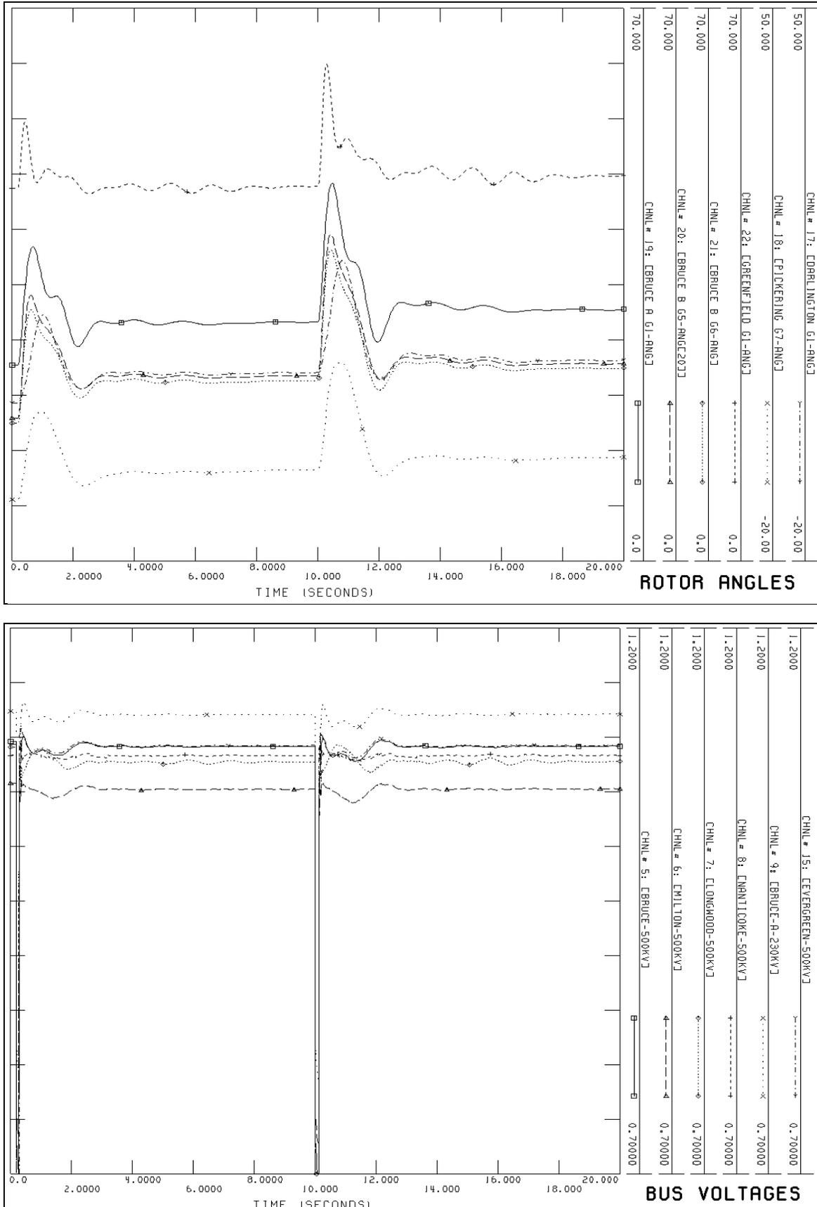
Figure 6: A563L & E562L – LLG fault @ Longwood with reclosure
