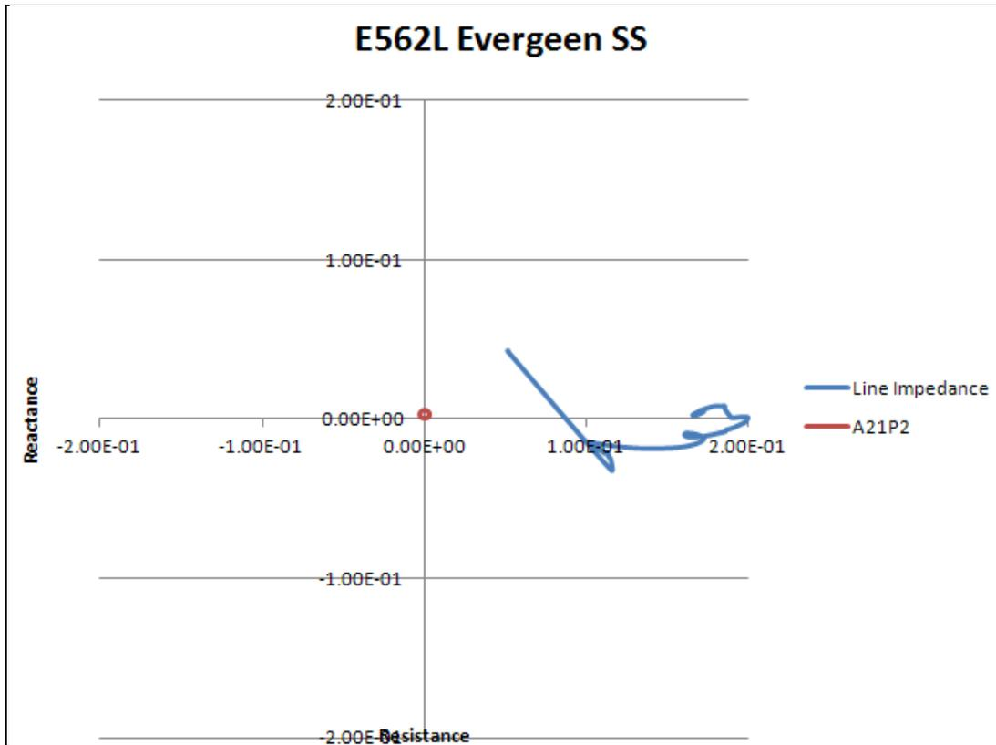
Figure 15: E562L @ Evergeen trajectory for a 3 phase fault on B563A at Bruce
