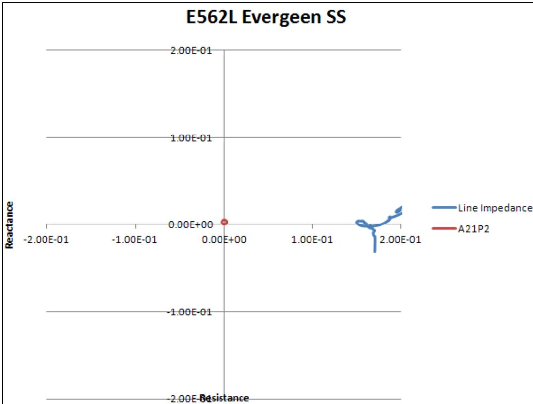
Figure 19: E562L @ Evergeen trajectory for a 3 phase fault on A563L at Longwood
