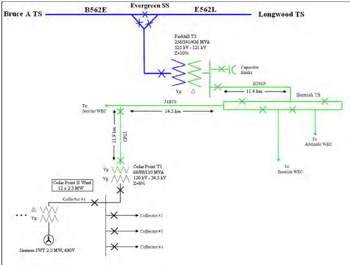
Figure 1: Cedar Point II Wind Power Project Single Line Diagram
