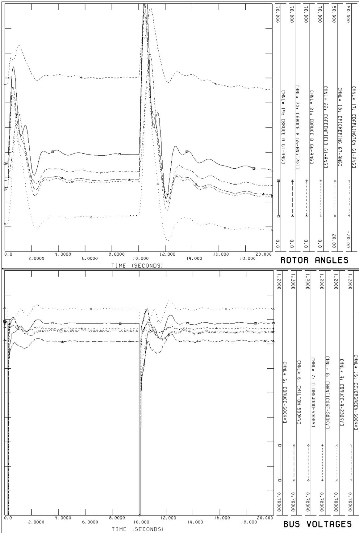
Figure 5: B562E & B563A – LLG fault @ Bruce with reclosure
