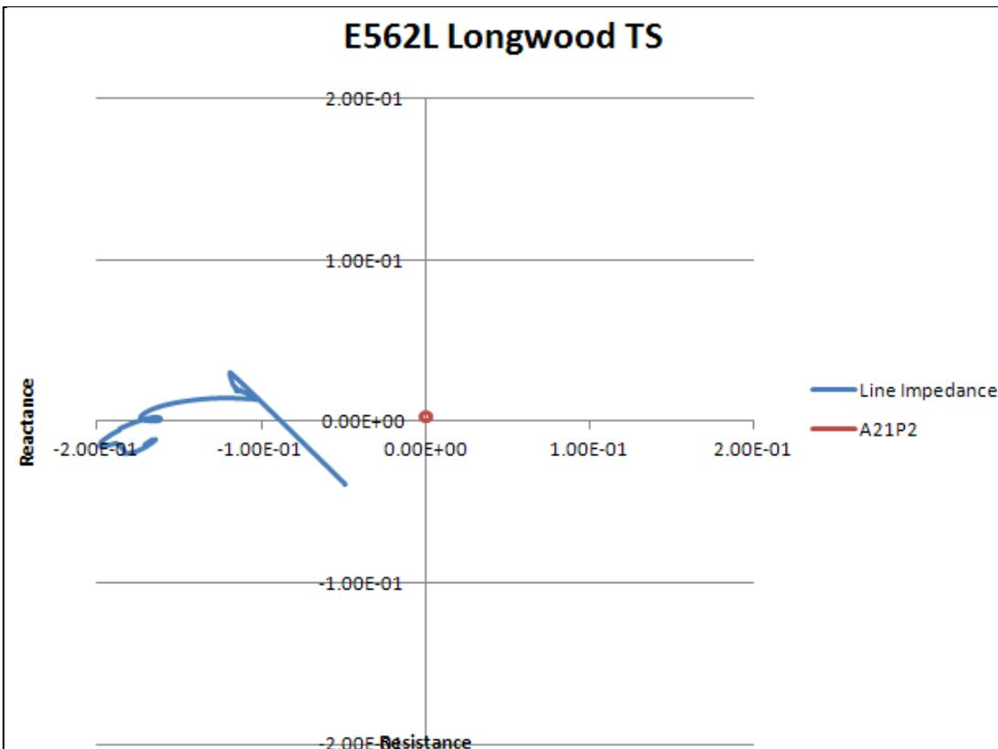
Figure 16: E562L @ Longwood trajectory for a 3 phase fault on B563A at Bruce
