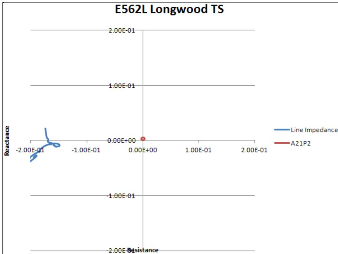
Figure 20: E562L @ Longwood trajectory for a 3 phase fault on A563L at Longwood
