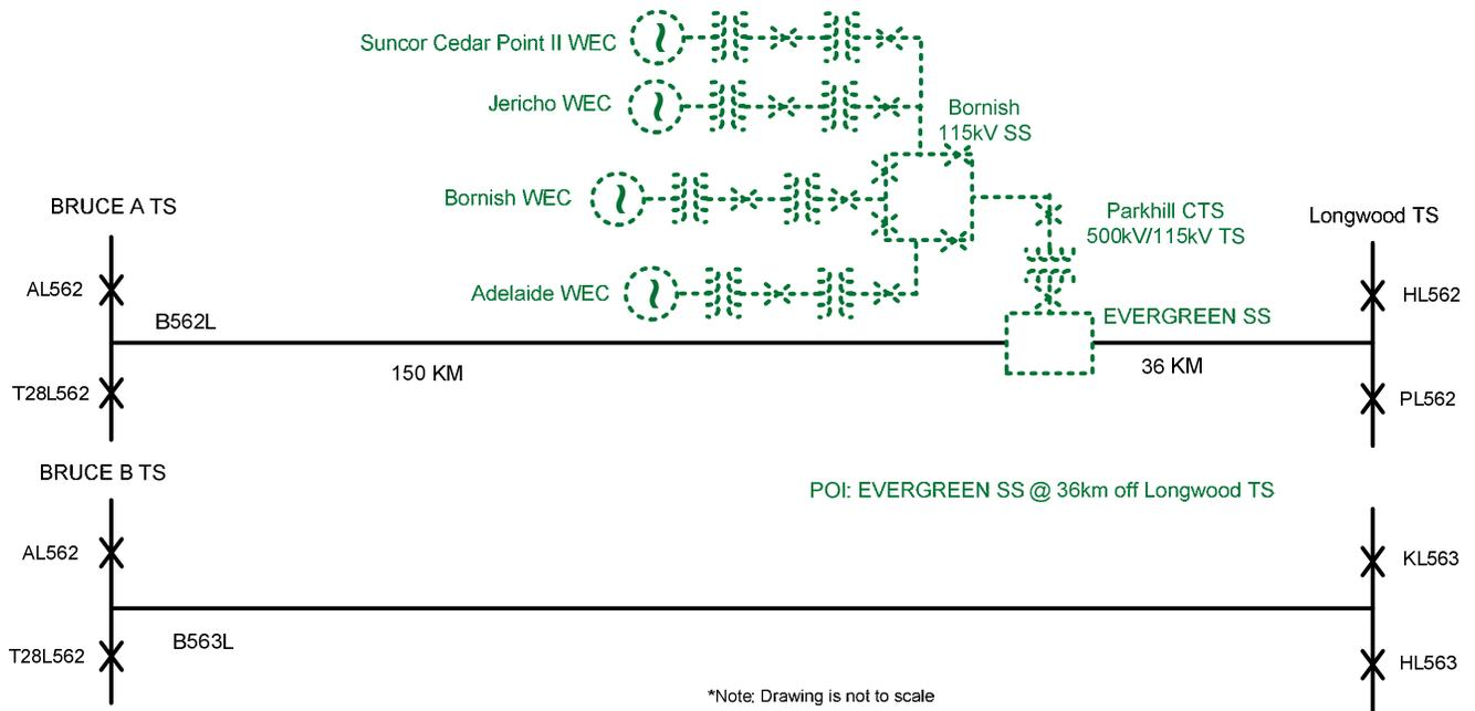
**Figure 1: NextEra/SUNCOR WF Connection to HONI Transmission System**
