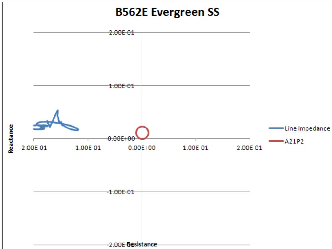
**Figure 10: B562E @ Evergreen trajectory for a LLG fault on B560V and B561M at Willow Creek Junction**
