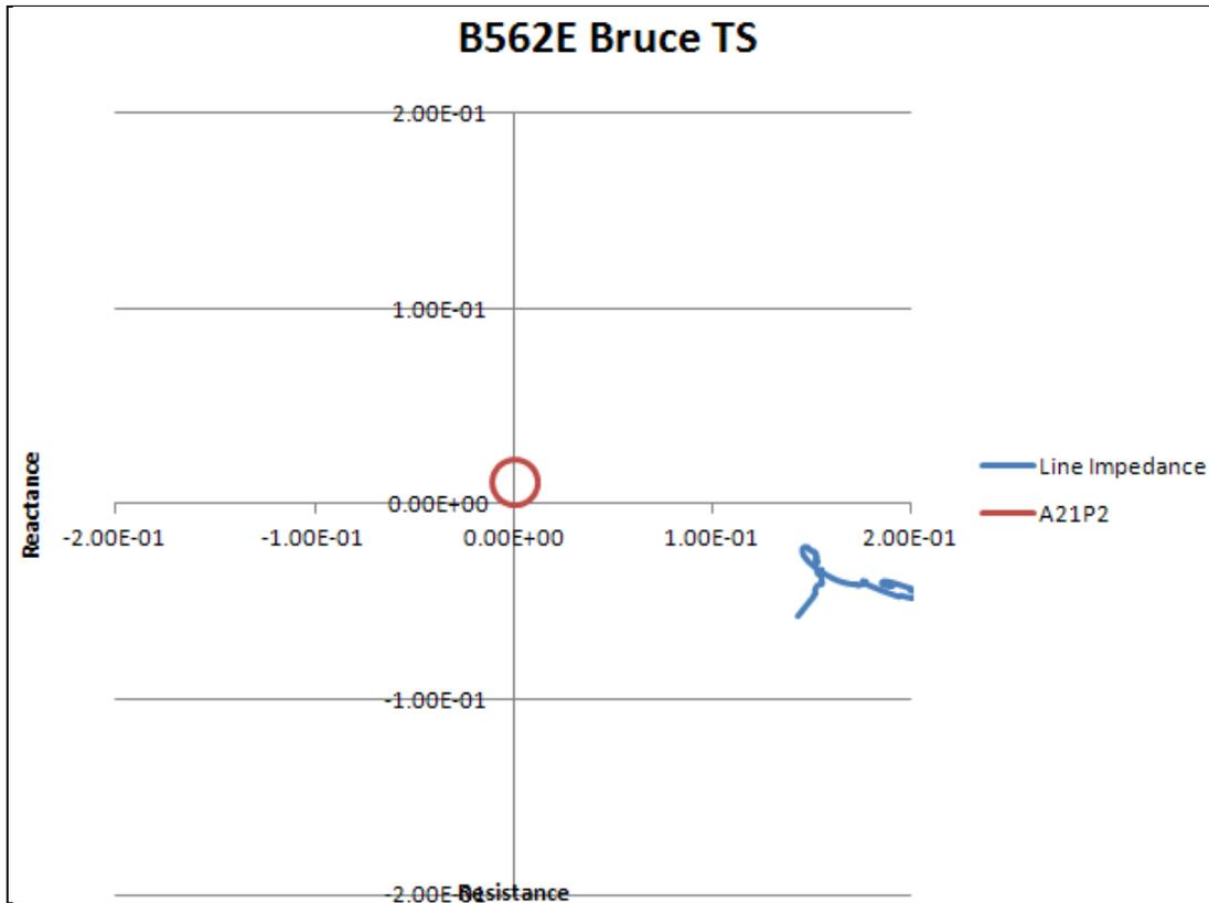
Figure 17: B562E @ Bruce trajectory for a 3 phase fault on A563L at Longwood
