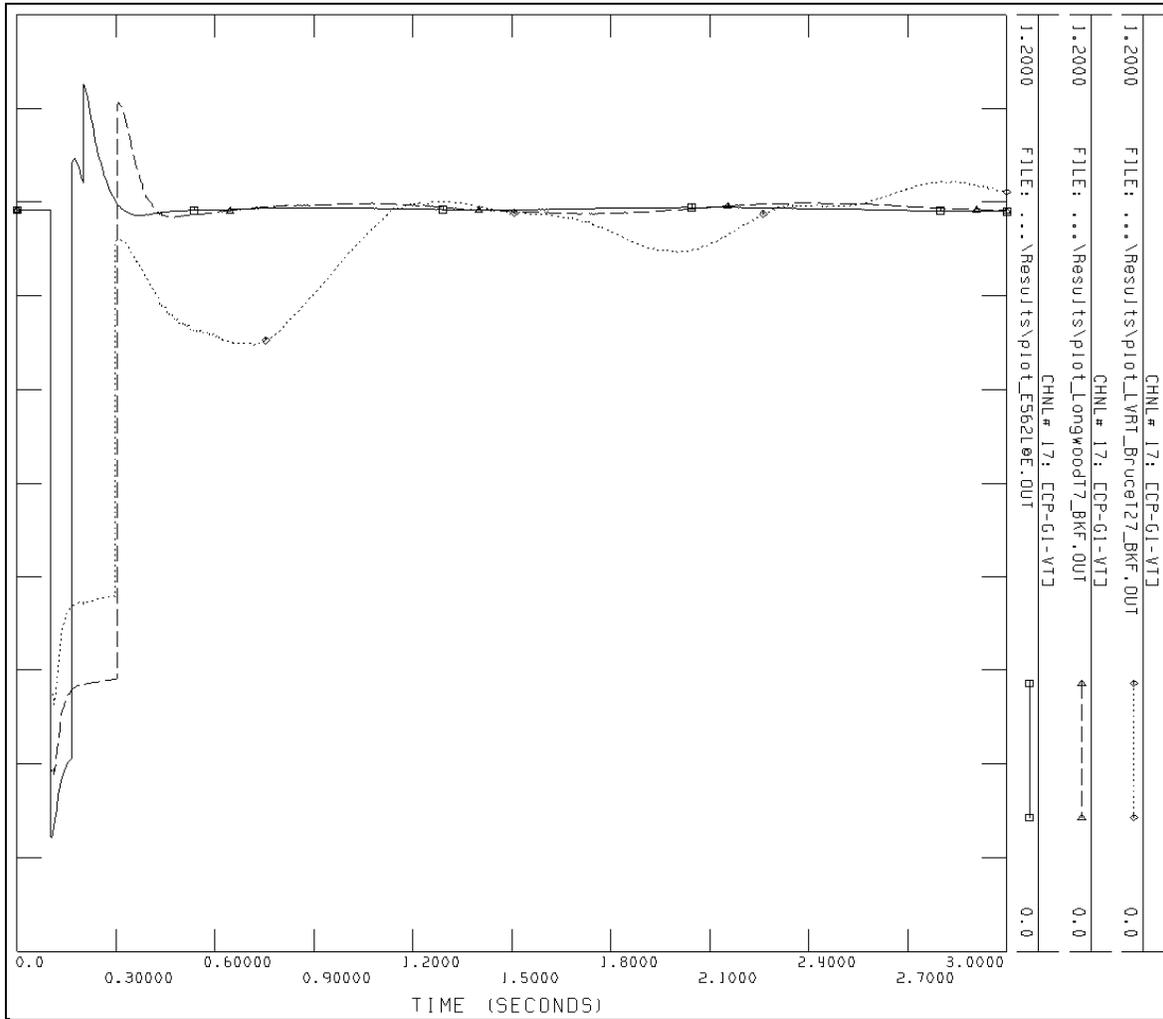
**Figure 8: WTG terminal voltages of feeder C1 for studied contingencies**
