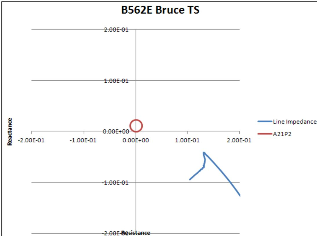
Figure 13: B562E @ Bruce trajectory for a 3 phase fault on B563A at Bruce
