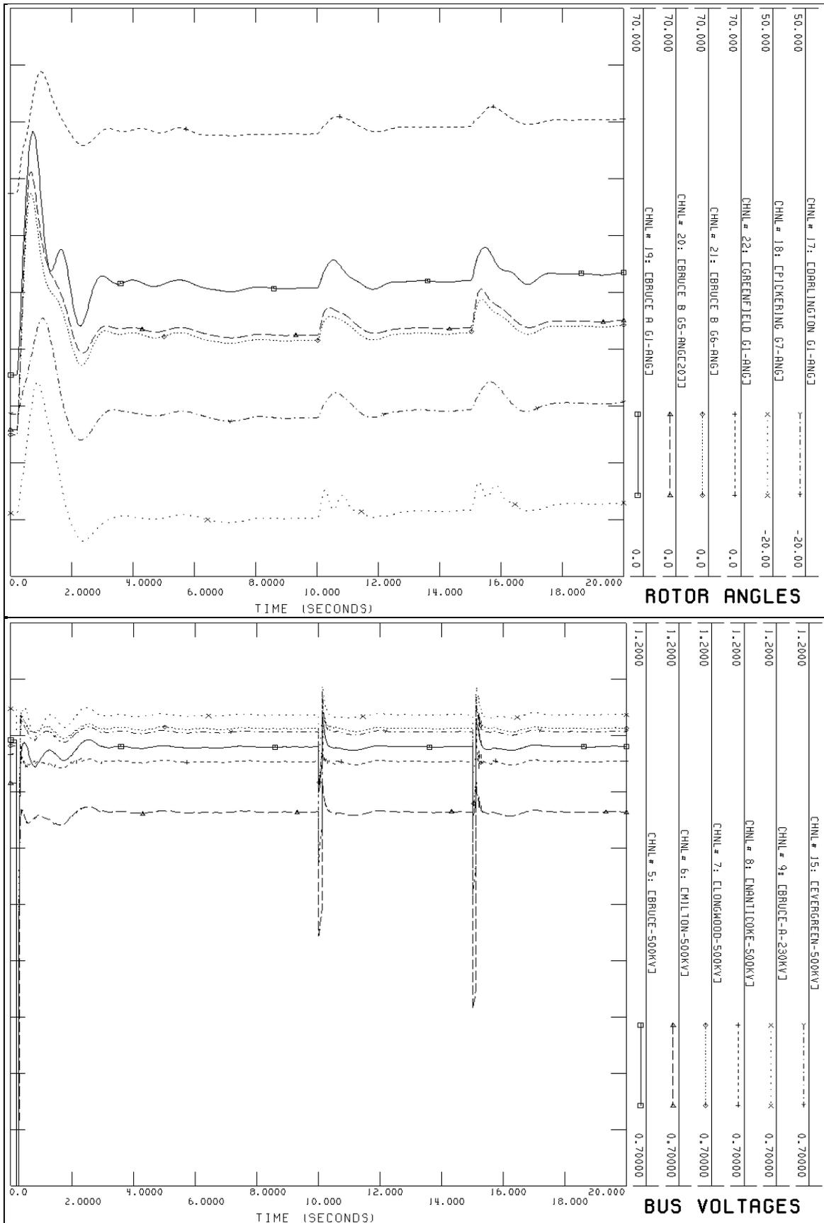
**Figure 4: B560V & B561M – LLG fault @ Willow Creek Junction with reclosure**
