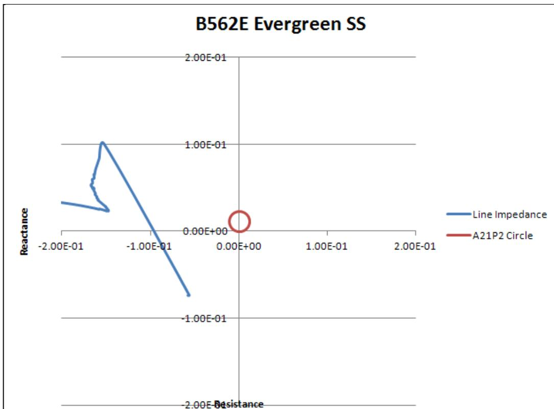
Figure 14: B562E @ Evergreen trajectory for a 3 phase fault on B563A at Bruce
