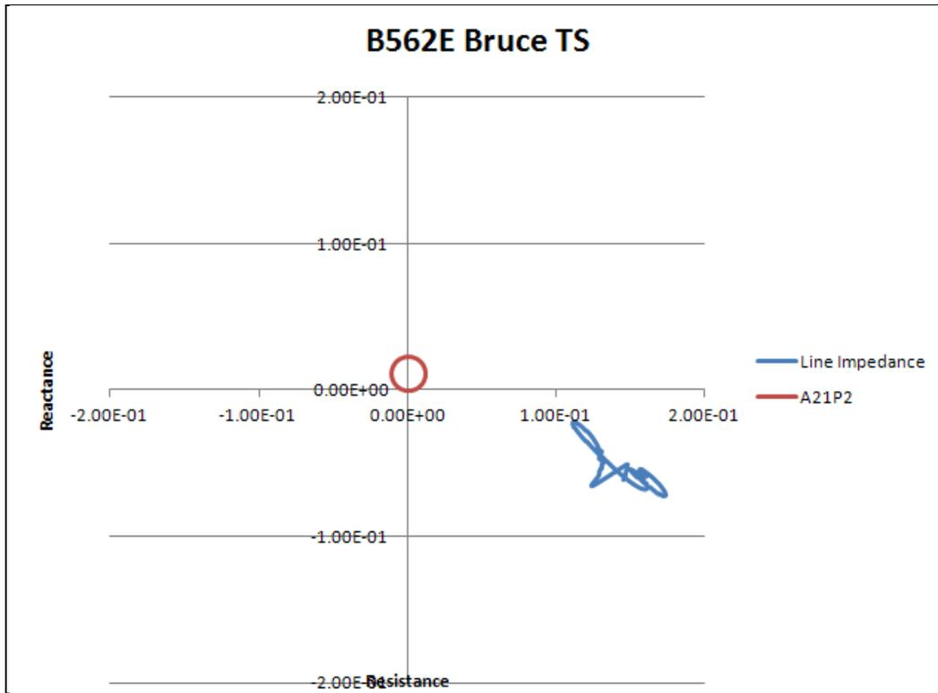
**Figure 9: B562E @ Bruce trajectory for a LLG fault on B560V and B561M at Willow Creek Junction**
