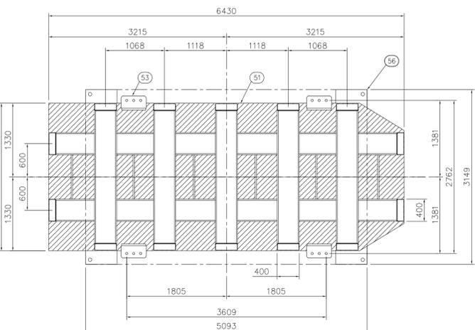
\* THE HATCHED AREA REPRESENT THE BOTTOM OF THE TRANSFORMER, THIS AREA IS NOT IN CONTACT WITH FOUNDATION OR PAD
