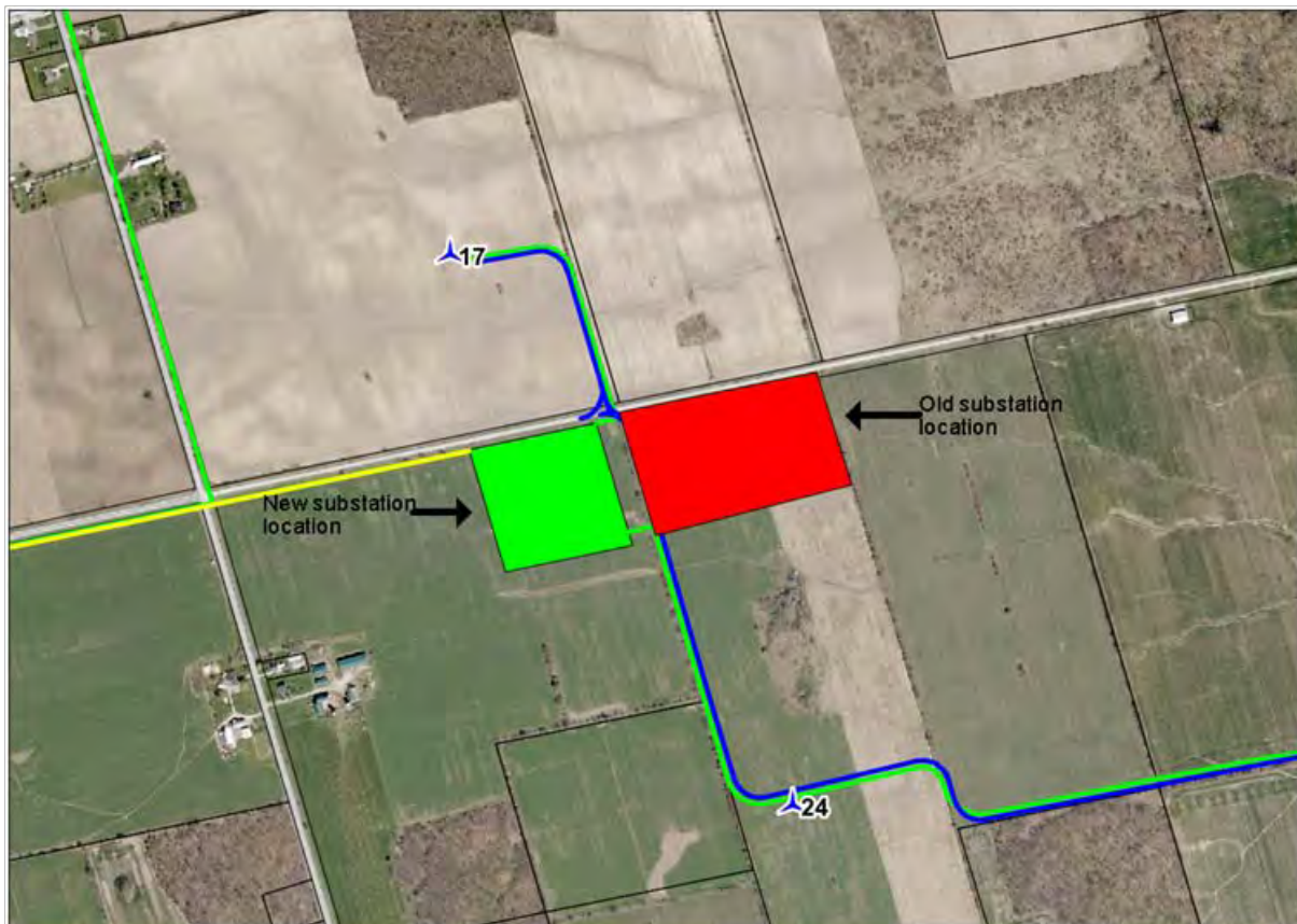
Figure 2: Aerial image showing the revised location and dimensions of the Project substation
