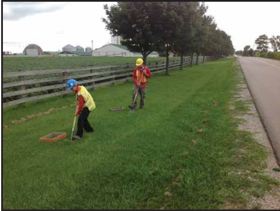
Image 173: View of Crewmembers Test Pitting to Confirm Disturbance at GSH2158 (Photo Taken August 13, 2013; Facing Northwest)
