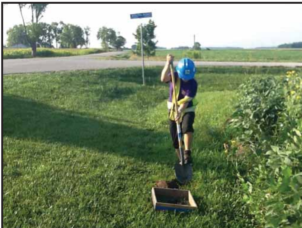
Image 208: View of Crewmember Test Pitting to Confirm Disturbance at Babylon Line from GSH2058 to GSH2030 (Photo Taken August 29, 2013; Facing South)
