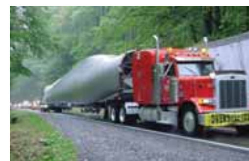
Blades are transported to the site for assembly with the wind turbine.
