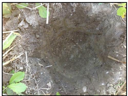
Image 84: View of Typical Test Pit Excavated 5 cm into Subsoil at GSH1095 (Photo Taken August 14, 2013)
