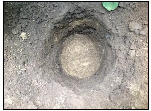
Image 21: View of Typical Test Pit Excavated 5 cm into Subsoil at GSH1023 (Photo Taken August 13, 2013)
