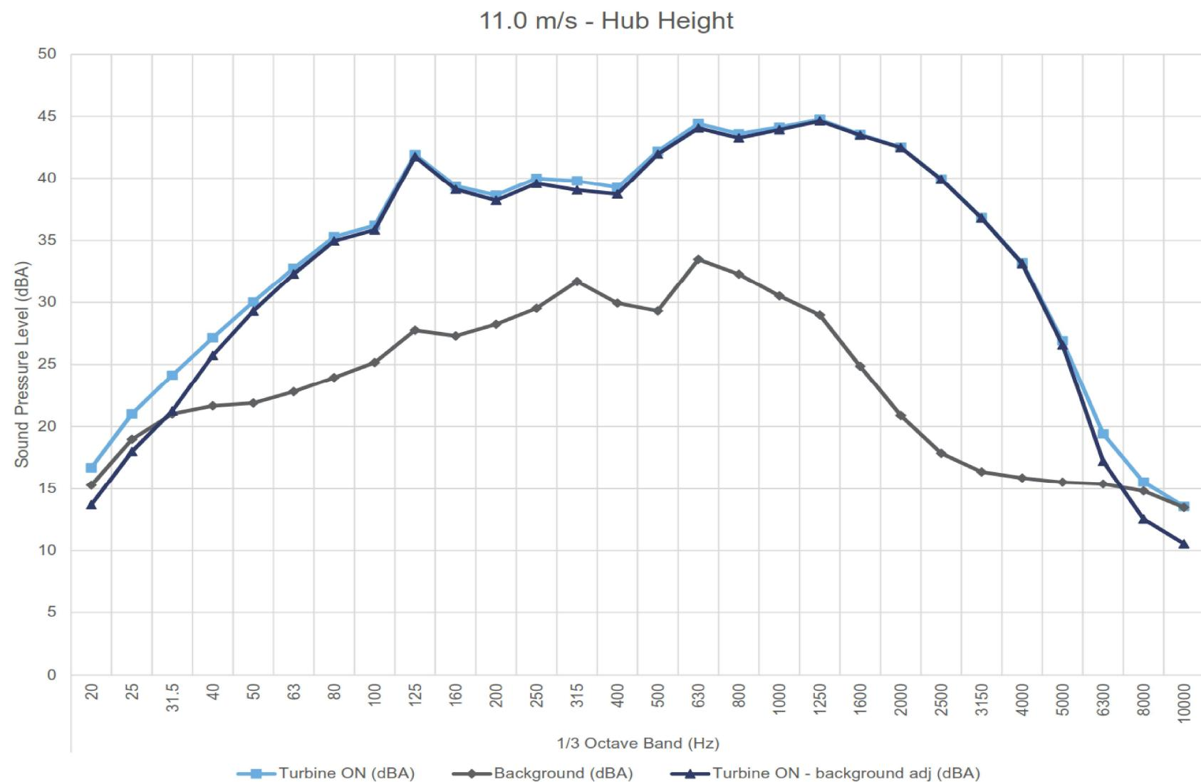
**Table C.01 Detailed apparent sound power level data at hub height**
