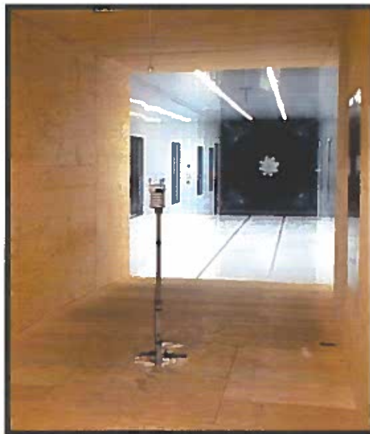
Photo of the wind tunnel setup. The cross-sectional area is 2.5 x 2.5 m.
