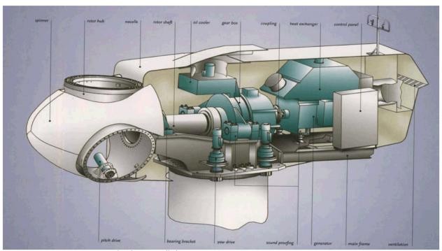
Figure 1: GE Energy 1.6-100 wind turbine nacelle layout
