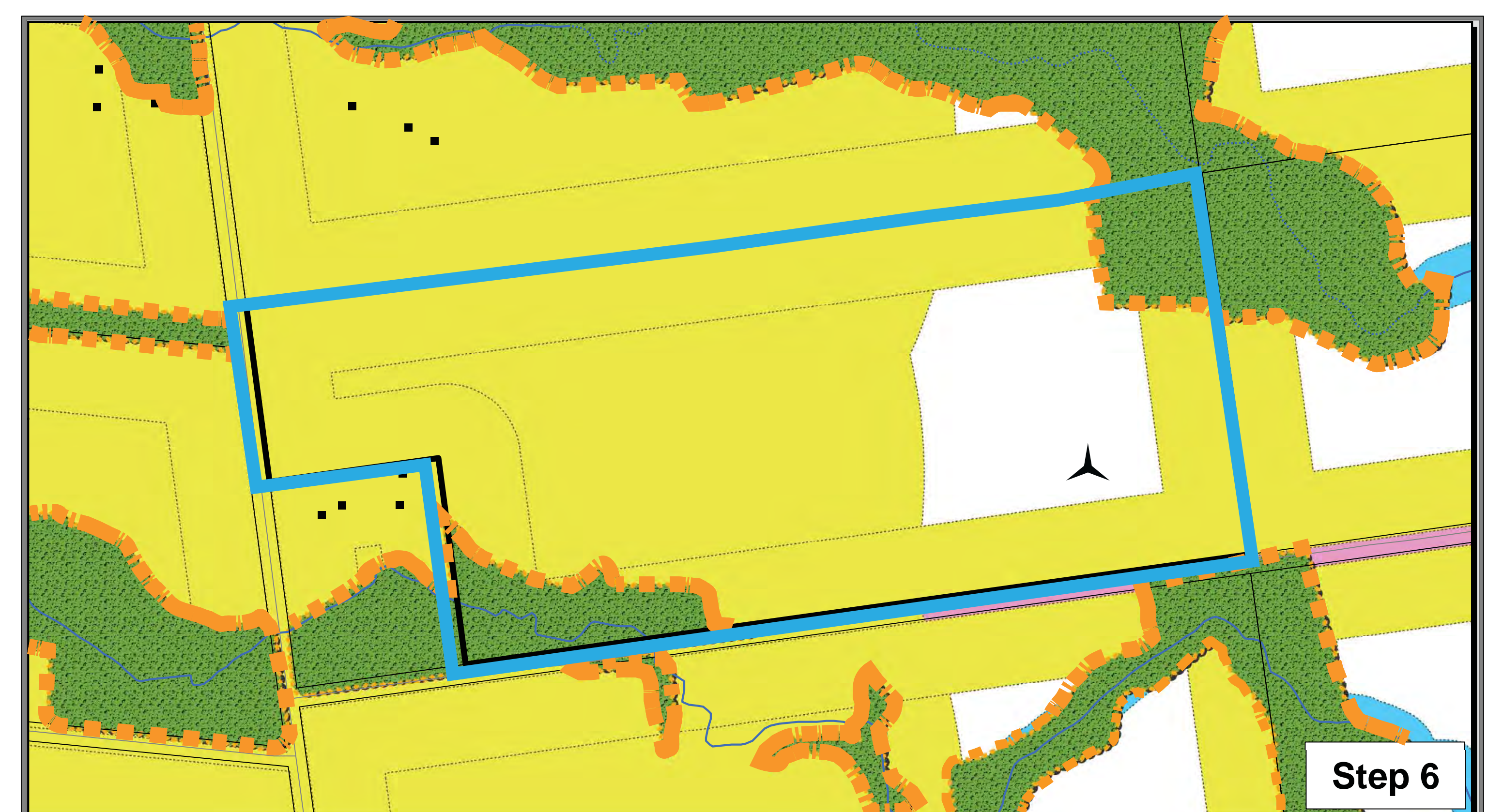
Step 6: Site turbine within remaining land available
