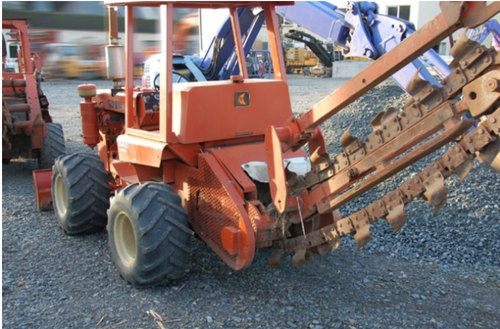
Figure 4.5-4: Example of a Cable Trenching Machine or “Ditch Witch”
