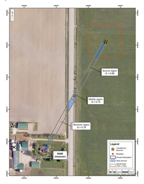
Figure 6-1: Ground factor coverage near Adelaide substation
