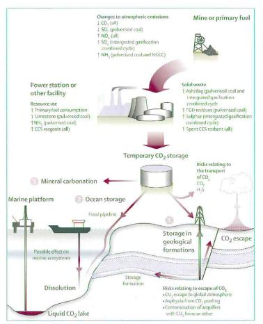
Figure 4: Summary of the principal CO, capture and storage processes and associated sources of environment and health risks
